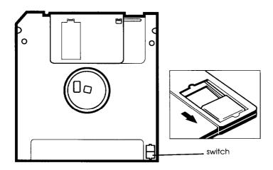
To remove the write protection, slide the switch toward the center of the diskette until it clicks into position and the hole is covered.
